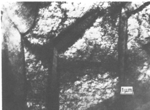
Figure 6 TEM of burst plates showing fine twins.
