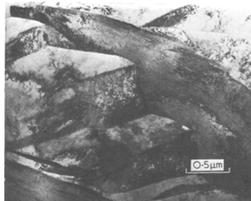
Figure 8 TEM of isothermal martensite showing branching of the chevrons.
