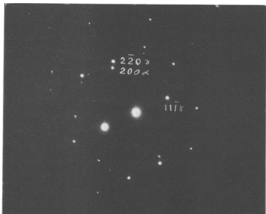
Figure 10 Selected-area diffraction taken from both austenite and martensite.
